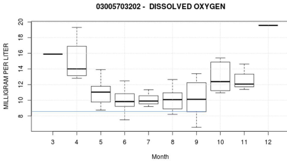
Figure 4-4 Dissolved Oxygen Concentrations Downstream of the Outfall Option
