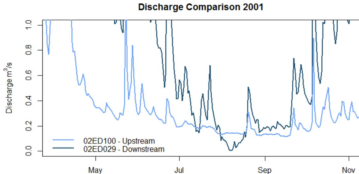
Figure 3-3 Base Flow Alteration by Extraction Example
