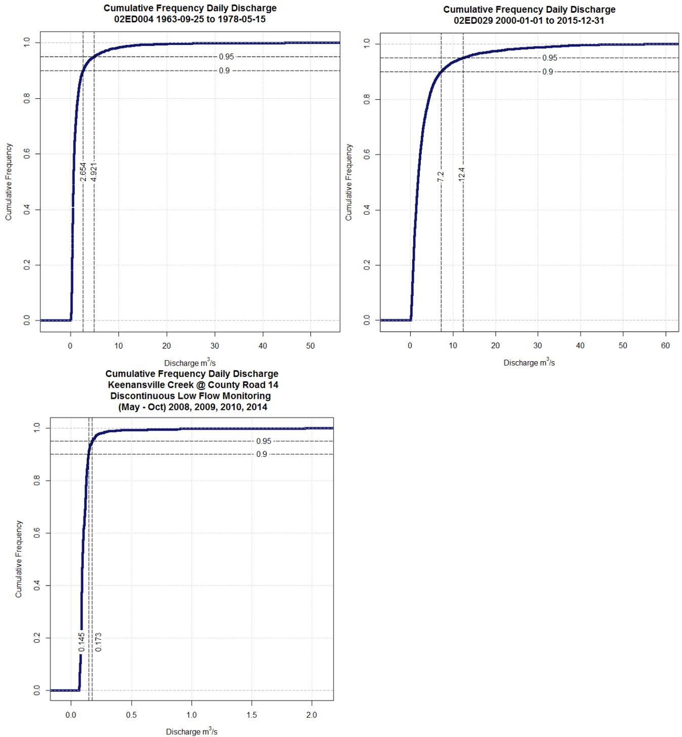
Figure 2 Cumulative frequency of discharge at WSC station 02ED004 (top left) and 02ED029 (top right), discontinuous low flow monitoring at County Road 14 (bottom).
