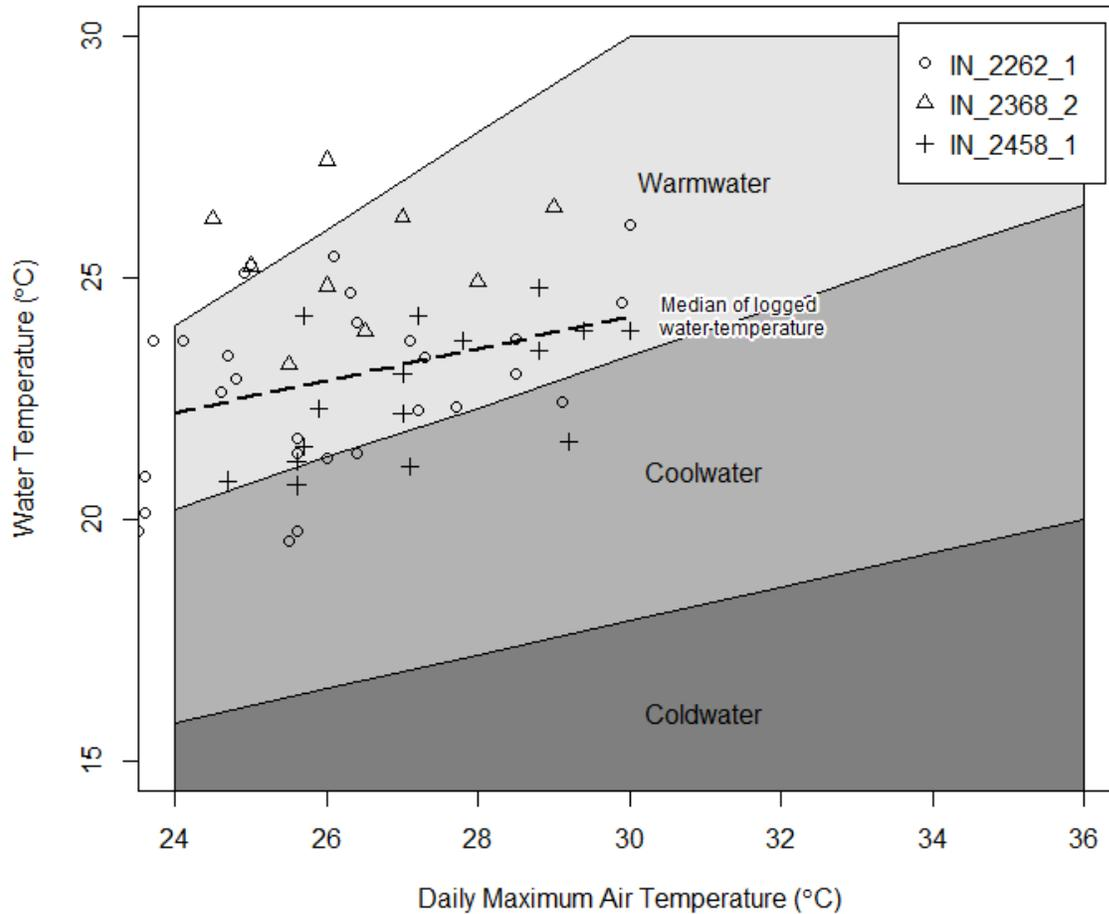
Figure 4-3 Stream Thermal Characteristic Nomogram, Adapted from Stoneman and Jones, 1996 with Overlay of Measured Data
