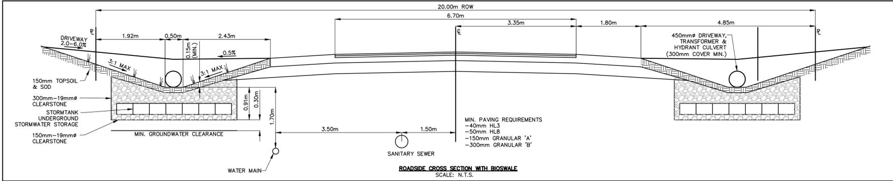
ROADSIDE CROSS SECTION WITH BIOSWALE
